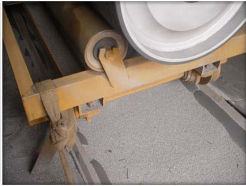
Standard Classic Conveyor idler rolls used in Shotblast Booth still turning freely after 1 year operation
